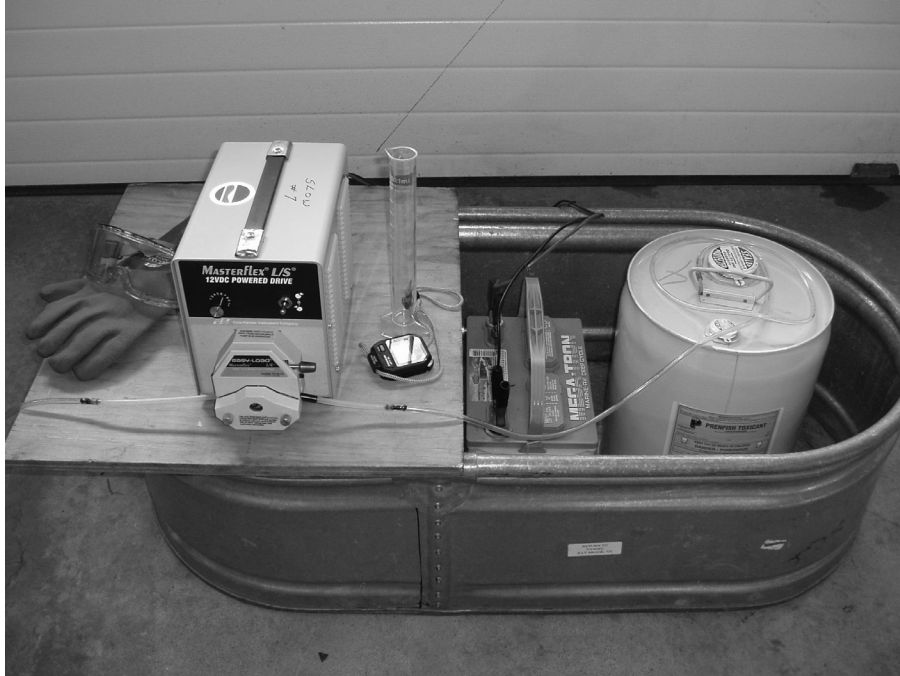
FIGURE SOP 11.1. Masterflex peristaltic pump set up in secondary containment area. Personal protective equipment, stop watch, and graduated cylinder are also shown.
