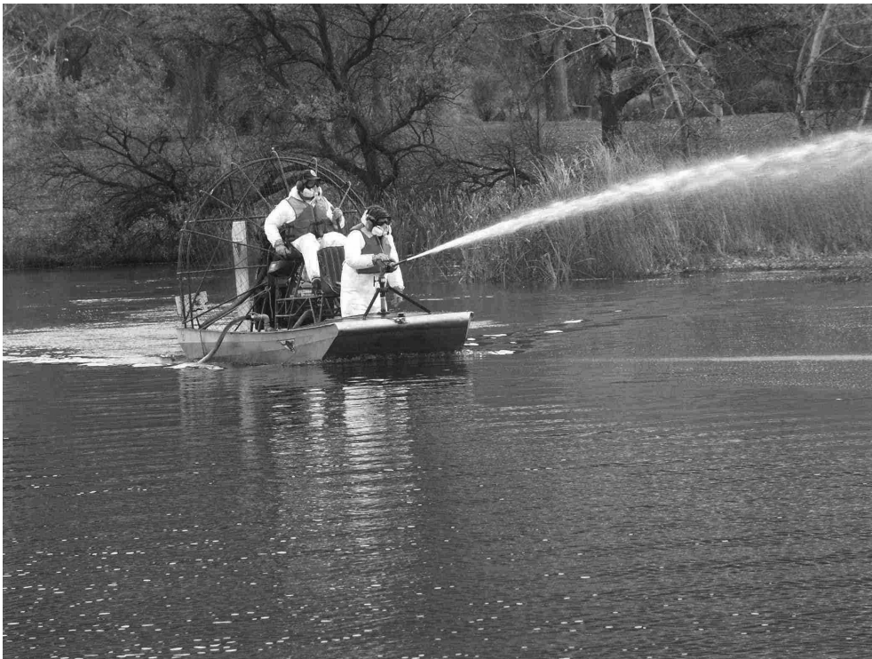
FIGURE SOP 8.6. Application of liquid rotenone using semi-closed application system with spray nozzle to shallow waters of Park Lake, Grant County, Washington (Photo credit, Jeff Korth, Washington Department of Fish and Wildlife).
