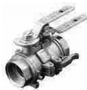
FIGURE SOP 8.4. An example of a dry disconnect valve showing the two halves coupled together with cam arms. Two interlocking handles make opening and closing easy. No guessing involved. When liquid is flowing, disconnect valve halves cannot be uncoupled without turning handles to closed position. When disconnect valve halves are apart, handles cannot be turned to open position.
