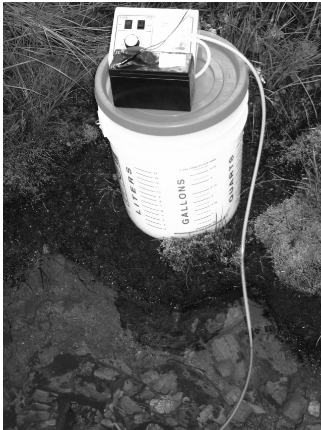
FIGURE SOP 11.2. Control Company peristaltic pump placed on rotenone bucket showing dispensing tube into stream. A 9-V battery sits alongside the pump.
