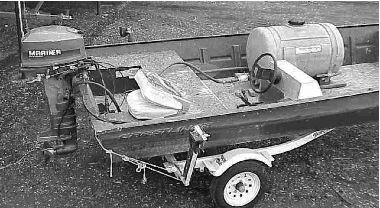
FIGURE SOP 11.3. Set-up of reservoir with pre-diluted liquid rotenone and venturi on small boat with out board motor.
