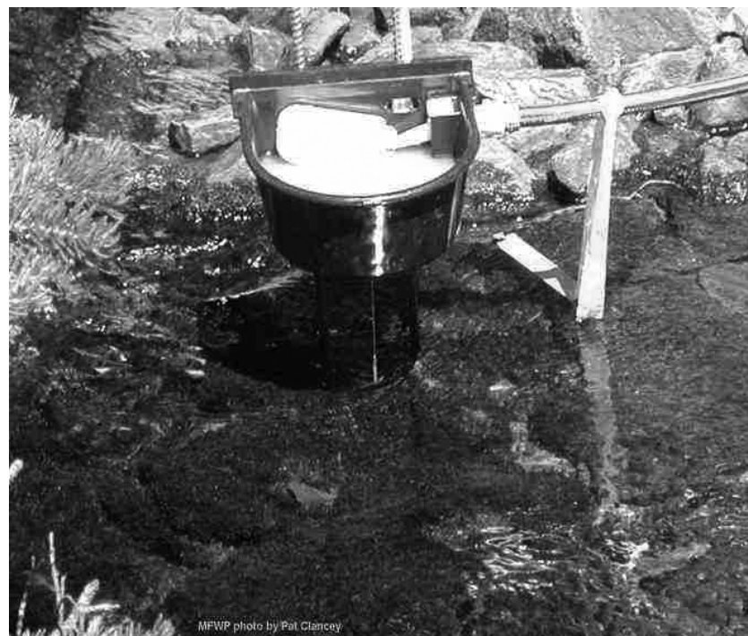
APPENDIX FIGURE 4. Dog watering bowl reservoir and float in operation.
