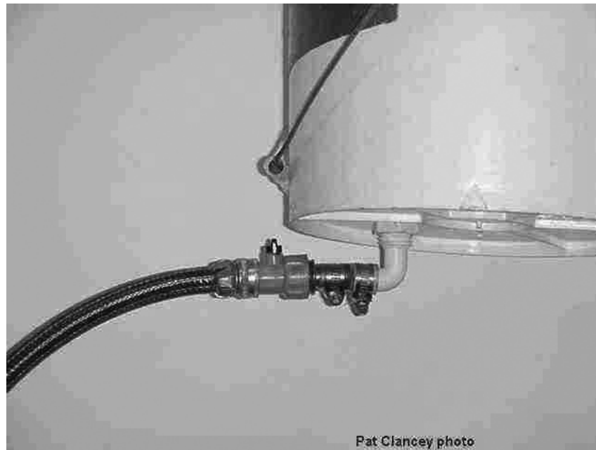
APPENDIX FIGURE 3. Drip bucket reservoir showing cut-off valve and garden hose attachment.
